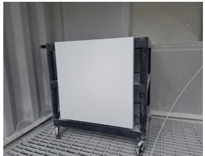
EFW Panel During Dust Ingress Testing
