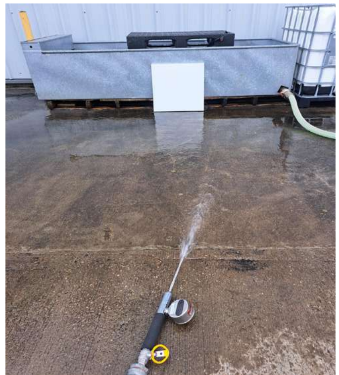
EFW Panel During Water Ingress Testing
