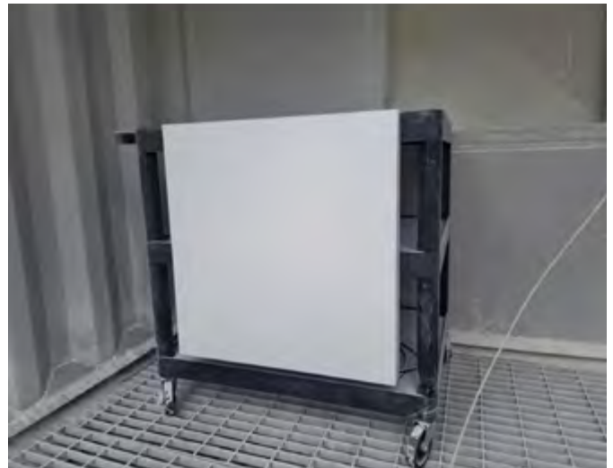
EFW Panel During Dust Ingress Testing
