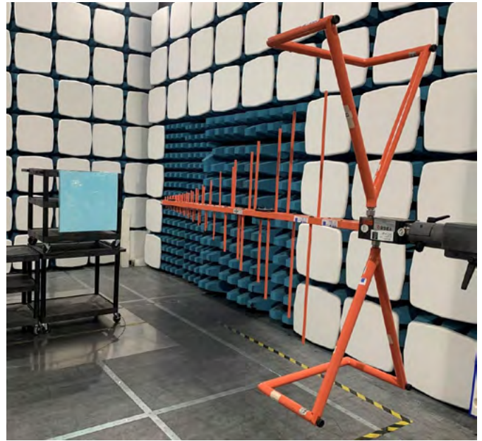
EFW Panel Electromagnetic Compatibility Testing - With a Chase CBL 6143A Antenna
