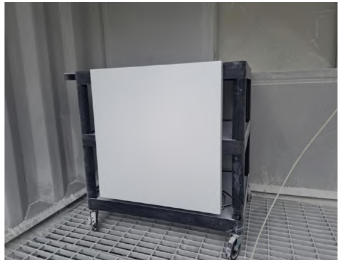
EFW Panel During Dust Ingress Testing
